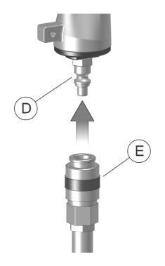
Connect the pneumatic marker to the compressed air pipe (E) by the quick nipple (D) in the lower part of the marker (see figure). During the use of the marker it is important to ensure that the supply air pressure never drops below 5 bar and does not exceed 8 bar. Use only filtered, lubricated and dried air; the use of any other power fuels such as compressed or flammable gas can cause explosions with danger for persons.
