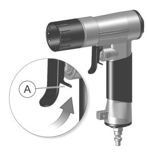
Before start any maintenance or exchange punches it is very important to disconnect the air supply pipe from the pneumatic marker. Then make sure to have turned up the safety device (A) behind the trigger (see figure). When the safety device is inserted the marking operation is locked.
